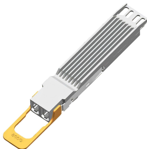
Figure 7.2.1 Dual MPO12 Module appearance
