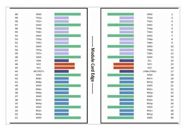
Figure 6.1 OSFP module pinout
